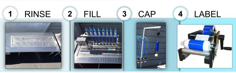
The Easy Fill is a great option for small businesses or for those who are looking to get started in the water bottling business. This unit uses premade bottles and incorporates bottle rinsing, filling, capping and rollon labeling. The bottling line can be operated by two to four people and is capable of producing up to 1,000 bottles per hour.
